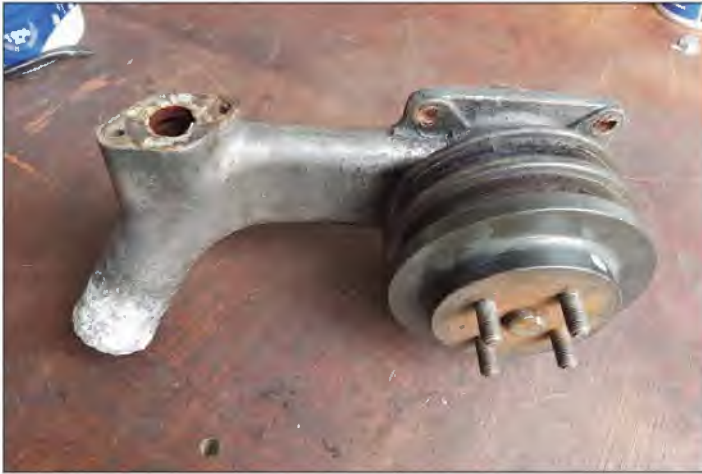
OLD WATER PUMP
